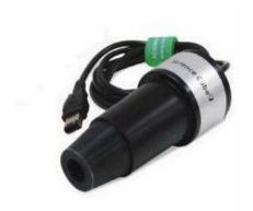
The Oxygen Gas Sensor measures the gaseous oxygen concentration in the range of 0
